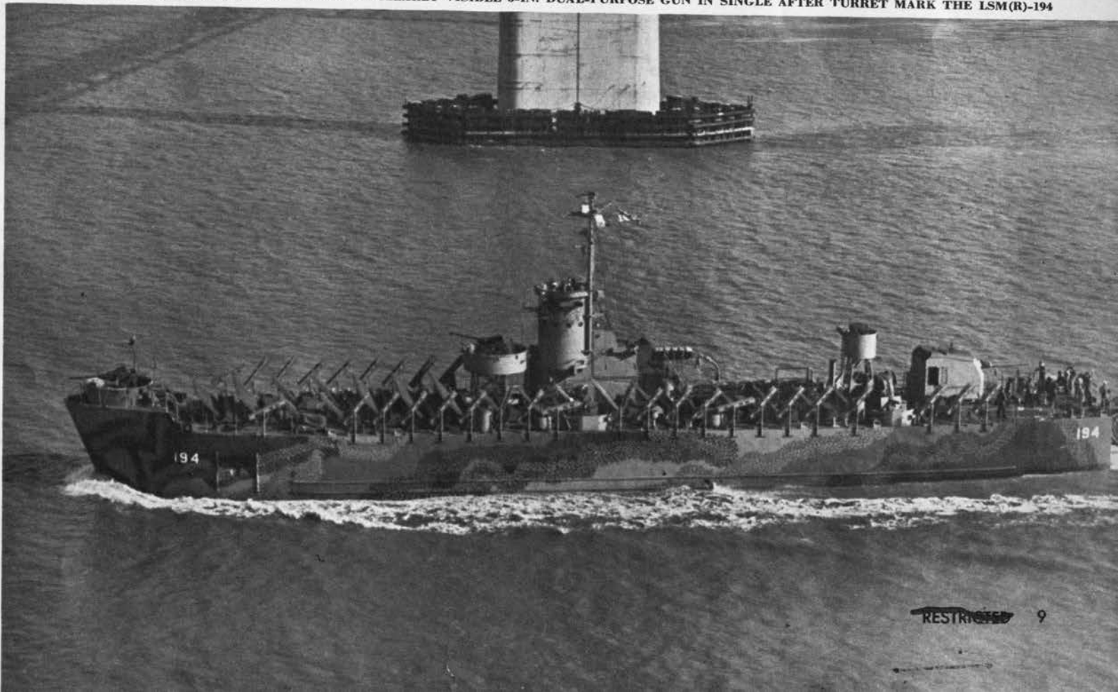
DECK CLUTTERED WITH ROCKET LAUNCHERS AND CLEARLY VISIBLE 5-IN. DUAL-PURPOSE GUN IN SINGLE AFTER TURRET MARK THE LSM(R)-194
